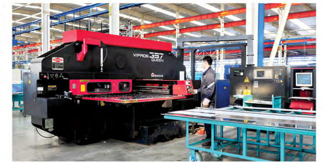
AMADA VIPROS-357Q Numerically Controlled Turret Punch Press
